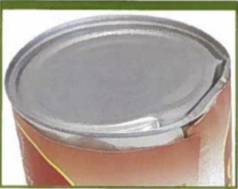
Severe dent in seam
